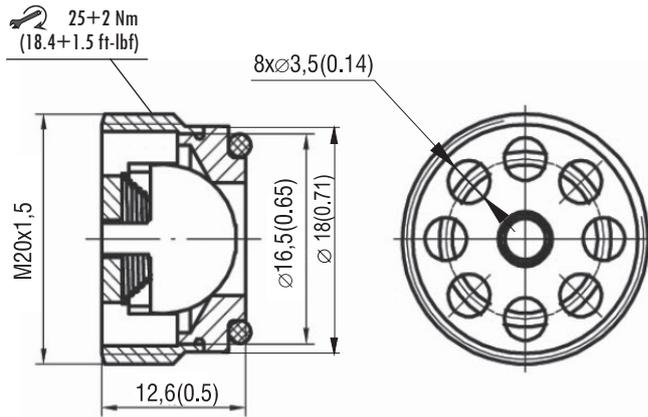
Tool for screwing the valve VJO1-10 into cavity
