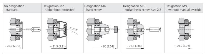
In case of solenoid malfunction or power failure, the valve spool can be shifted by manual override under the condition that the pressure in the back line does not exceed 25 bar (363 PSI). For alternative manual overrides contact our technical support.
