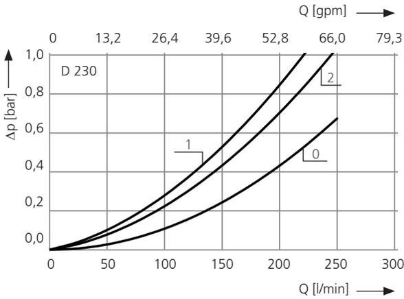
Pressure drop as a function of the **kinematic viscosity** at nominal flow
